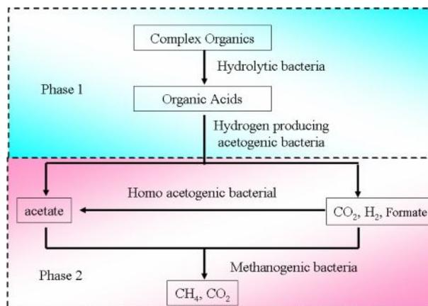
**Fig. 2 The two-phase anaerobic digestion system.**
