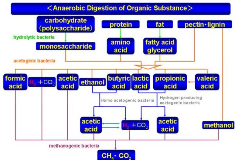
Fig.1 Methane fermentation scheme.
