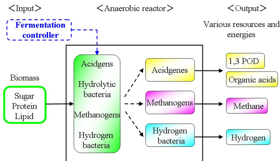
**Fig. 3 Novel bioprocess concept. Various resources and energies production.**
