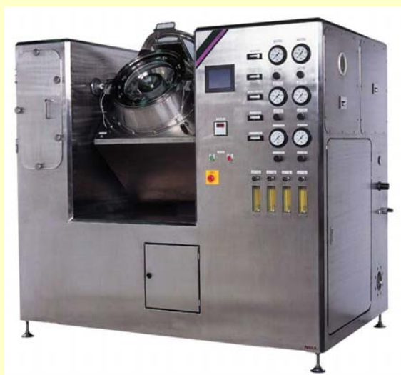
Novel nanoparticle fluidization device for granulation and film coating using a centrifugal field
